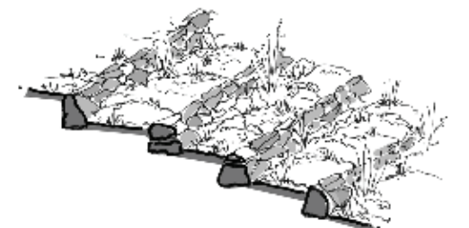
Natural rock walls are preferred for retaining
